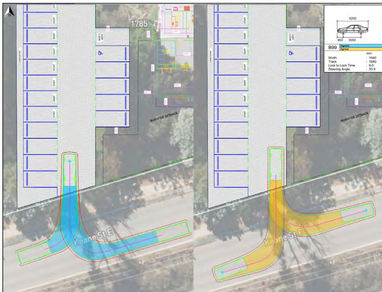
Figure 5-1 Sweep Path – Site Access
