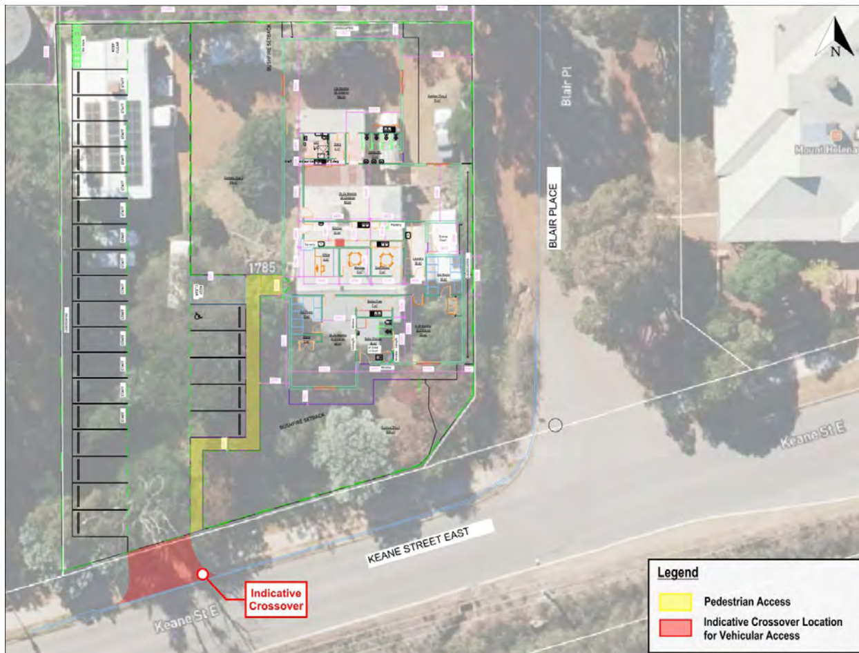
Figure 4-2 Site Access Arrangement
