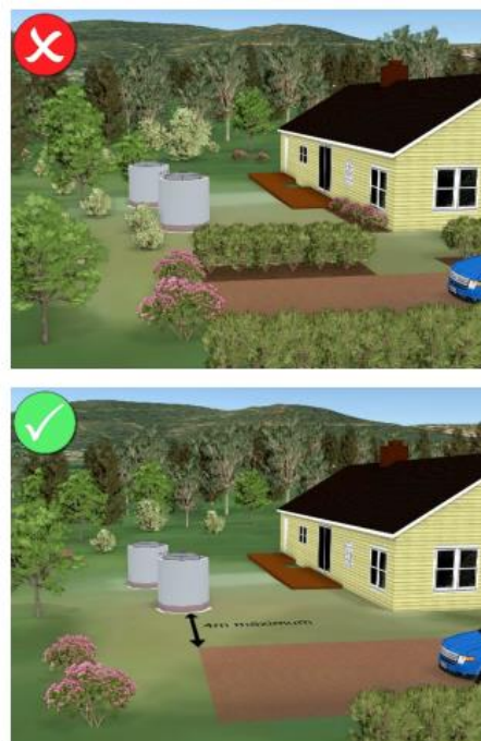
Figure 39: A good and bad example of landscaping around a water tank
