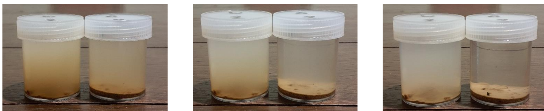
Figure 4.10 Dispersion and gypsum responsiveness TP2. In each photo the RHS jar is soil in gypsum solution. LHS jar is soil in water. (L set) after 15 minutes, (M) after 2 hours, (R set) after 20 hours.
