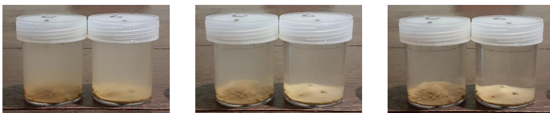
Figure 4.3 Dispersion and gypsum responsiveness TP1. In each photo the RHS jar is soil in gypsum solution. LHS jar is soil in water. (L) after 15 minutes, (M) after 2 hours, (R) after 20 hours.
