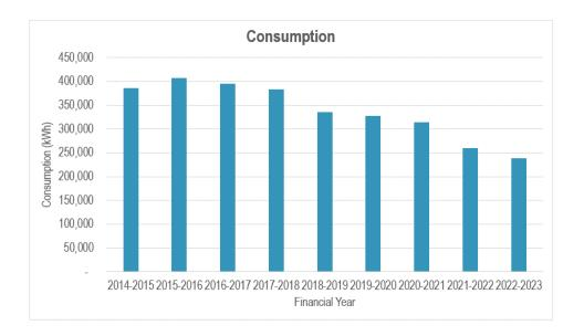
Shire of Mundaring Administration Centre – reducing energy consumption with improved energy efficiency through introduction of night purging and other improvements to air conditioning, changes to LED lighting, and other improvements to energy efficiency of equipment.
